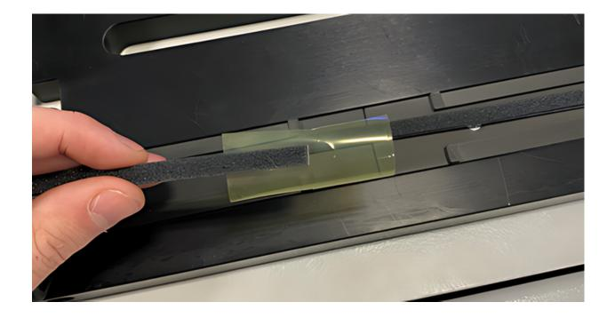
**4)** Peel back the material or adhesive foam on the trailing end and place the Leading end liner overlapped approximately 10mm (3/8"). The overlap in this direction is critical.
